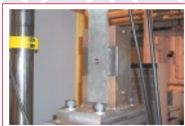
Single-lap joint with single fastener-specimen test setup (courtesy DERA)
