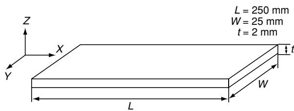
Fig. 5 Schematic draw and dimensions of the laminate.
