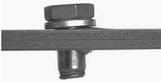
Fig. 8. Final failure of protruding head bolt.
