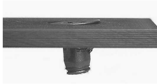
Fig. 9. Final failure of countersunk head bolt.
