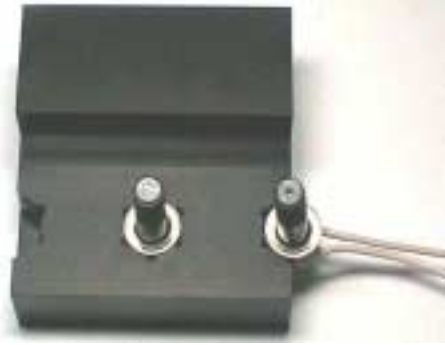
Fig. 4 Multi-bolt joint assembly jig used in the instrumented bolt tests to simultaneously centre the bolts in the holes, align them with the loading direction, and torque them to the required level
